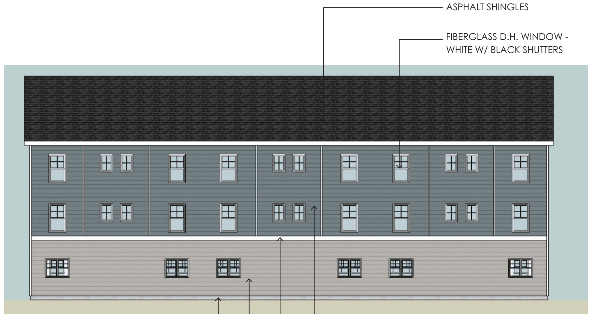
BUILDING #2 ELEVATION REAR ELEVATION
